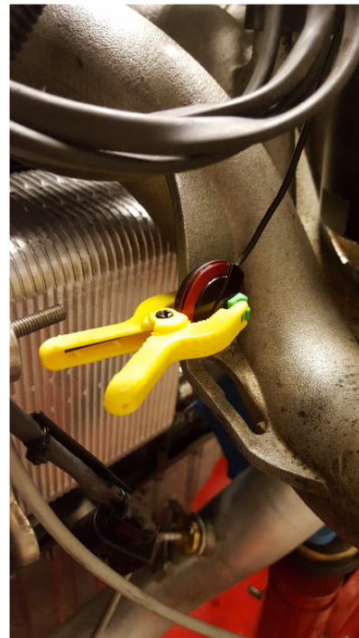
(b) Placement of microphone #1. A clamp keeps the microphone in place.
