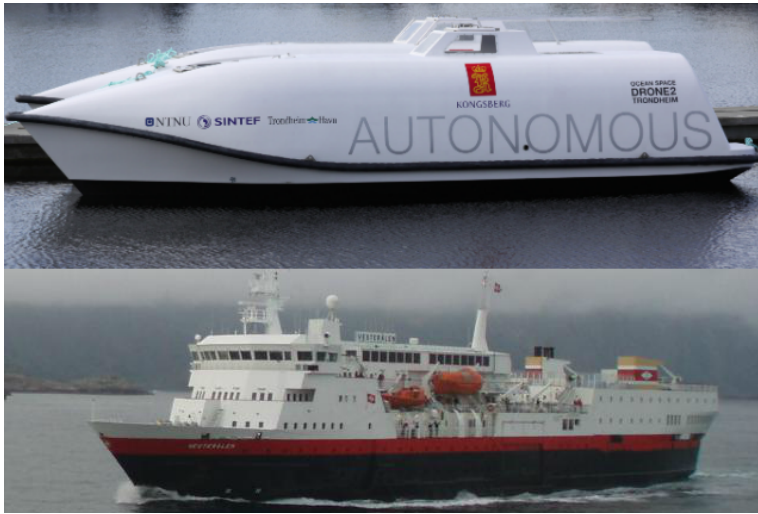
Figure 5.4: The two targets present in the scenario. The top is labeled ‘KSX_OSD1’ and was the target of a coordinated COLAV experiment, the bottom is a passing ferry labeled ‘Vesteraalen’.
