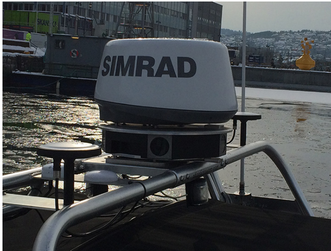
Figure 5.1: The radar used to obtain measurements for the scenarios ‘Seatex Drone’ and ‘Near Munkholmen and Approach’.
