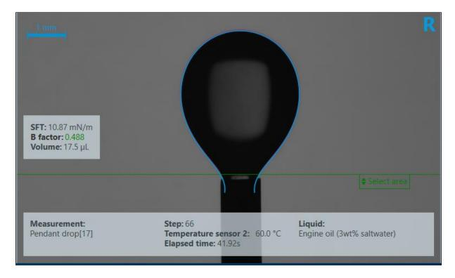
*Figure 23: Measuring the IFT between engine oil and synthetic brine at 60 °C*
