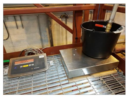
Figure 26: Weight connected to LabView
