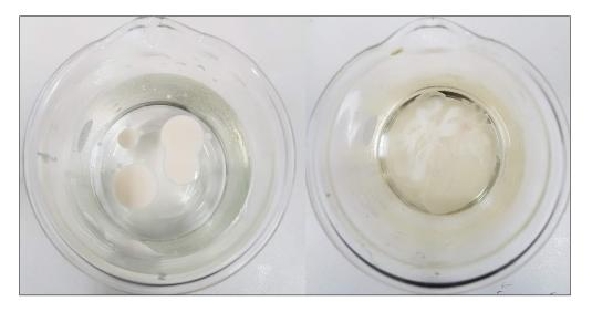
Figure 14: Pictures of the drop test. To the left, clearly defined drops of emulsion in water. To the right, same emulsion dissolving in soy oil.
