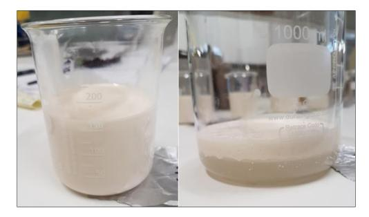
*Figure 13: Emulsions after mixing. To the left: W30-O70 emulsion shortly after mixing. To the right: W70-O30 emulsion shortly after mixing. One can clearly see that the emulsion has separated in to two distinct layers.*
