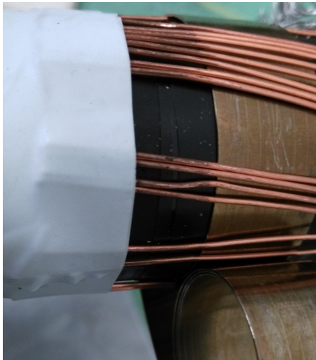
(a) Oxide layer on copper wires.
