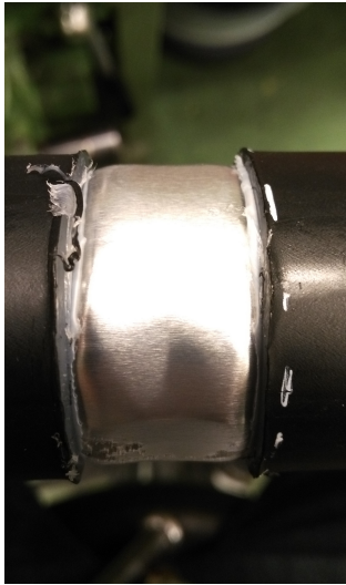
(a) Picture showing how the laminate was lifted when the outer sheath was removed.
