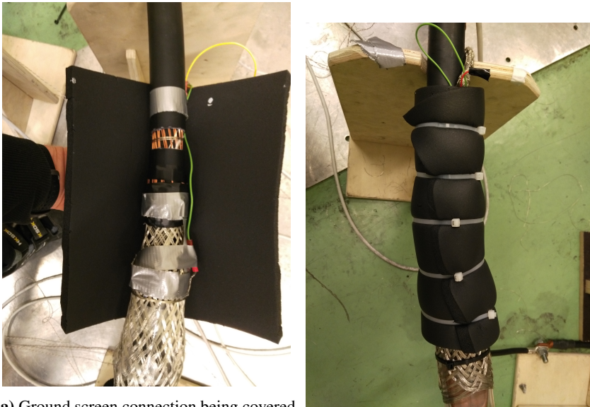
(b) Ground screen connection and measuring points wrapped in Armaflex, held in place by cable ties.
