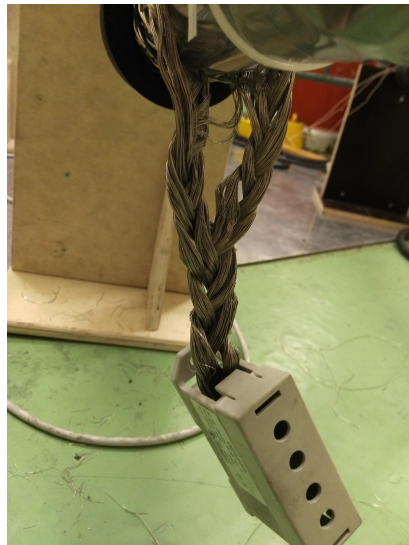
(b) Picture showing the connection of the braided joint ground screen to a terminal for interconnection.
