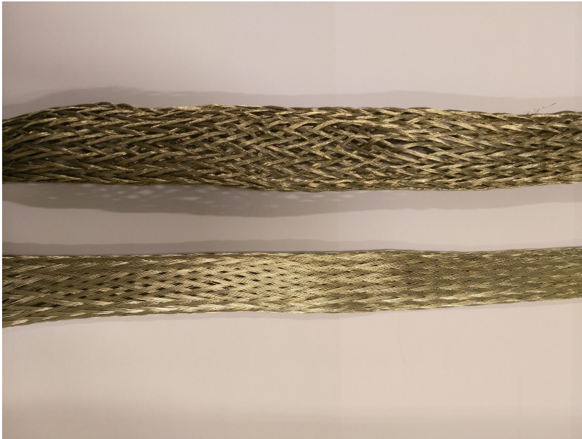
Figure 3.14: Figure showing the joint ground screen supplied with each ground screen connection type. On the top: type I, on the bottom: type II. It can be seen that type I is rougher than type I. Type II is more compressed when delivered than type I.
