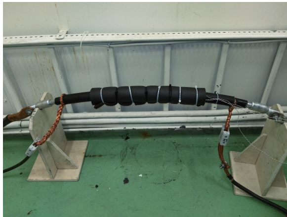
Figure 3.4: Picture of a finalized reference object, with thermal insulation applied. Screen and conductor connections can be seen on the cable ends. In addition the thermocouples are seen on the right side.
