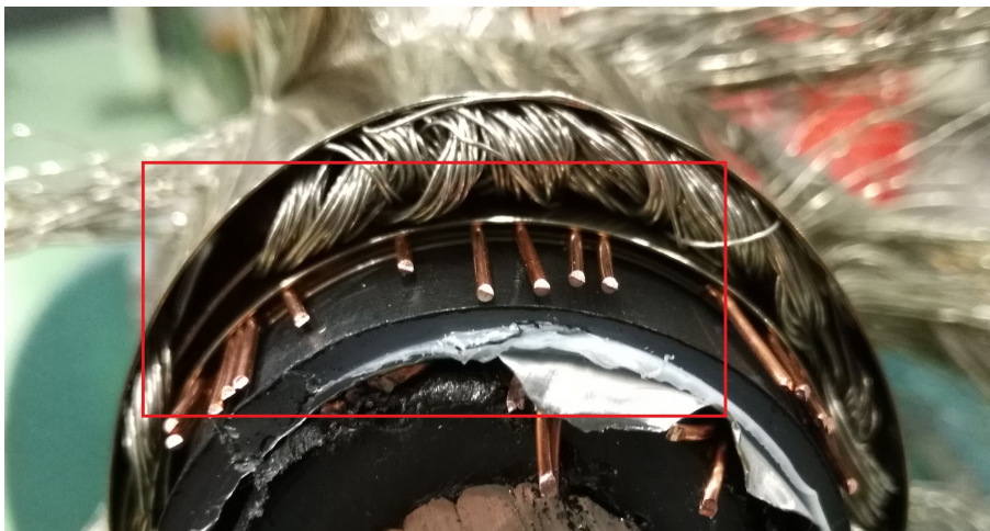
Figure 3.11: Picture showing the cross section of an incorrectly installed ground screen connection of type I. The cross section is taken from what would be the cable side of the joint in an installation. It can be seen that the copper wires and the joint ground screen is separated by a layer of the force spring (red box).
