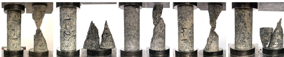
Figure 4.24: Pictures before and after testing showing failure mode
