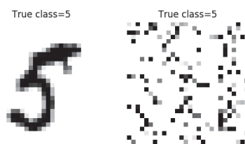
Figure 3.1: Example digit from the MNIST dataset [34]. Left and right images are identical except that pixels on the right have been randomly permuted. Applying the same permutation on all instances in the MNIST dataset and training a fully-connected network on it, will yield identical classification performance as on the original dataset.
