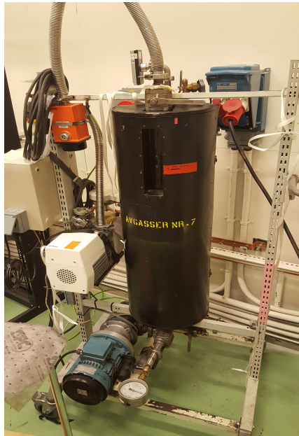
Figure 4.7: Photograph of the setup used for degassing the oil consisting of a container (black), heating elements, pressure pump (blue) and vacuum pump (white).
