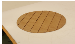
(a) Illustration of a bulk oil stack seen from the side. (b) Photographs of a butt gap stack with 7 butt gap sheets without an unmodified paper sheet on top.
