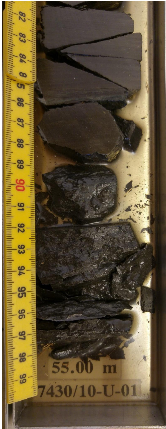
Figure 2: Example of the broken up parts of core 7430/10-U-01 at depth 54.90 m
