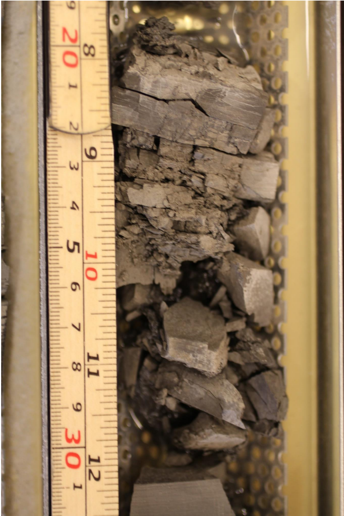
Figure 19: Massive mudstone at depth 152.20, from core 7018/05-U-01. This also shows how broken up the core is in some places.
