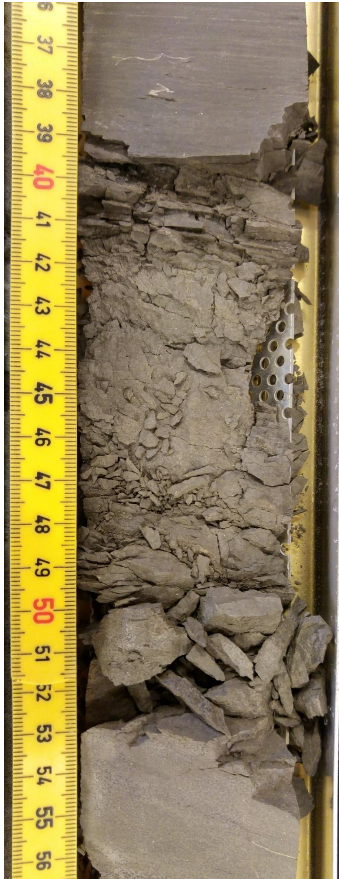
Figure 3: Example of broken parts of core 7018/05-U-01 at depth 65.40 m
