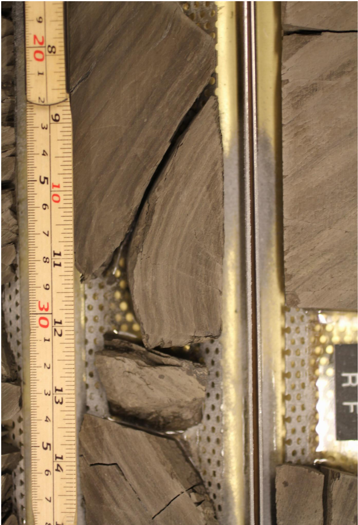
Figure 22: Close-up of slumping at depth 106.25m in core 7018/05-U-01. Lamination can be seen turning and going vertically down the core and bending within the layer.
