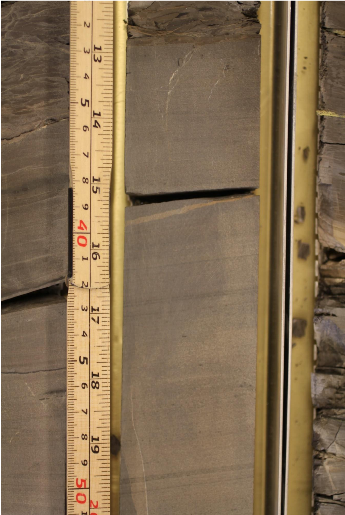
Figure 16: Siltstone at depth 217.74 from core 7018/05-U-01. The colour change towards the bottom might be a result of siderite cement, as there is a more massive layer of siderite cement just below this facies, also represented in the magnetic susceptibility data.
