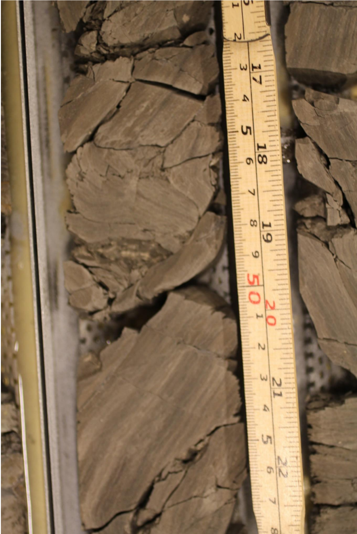
Figure 21: Close-up of slumping at depth 104.70 m in core 7018/05-U-01. Lamination can clearly be seen bending without being broken up.
