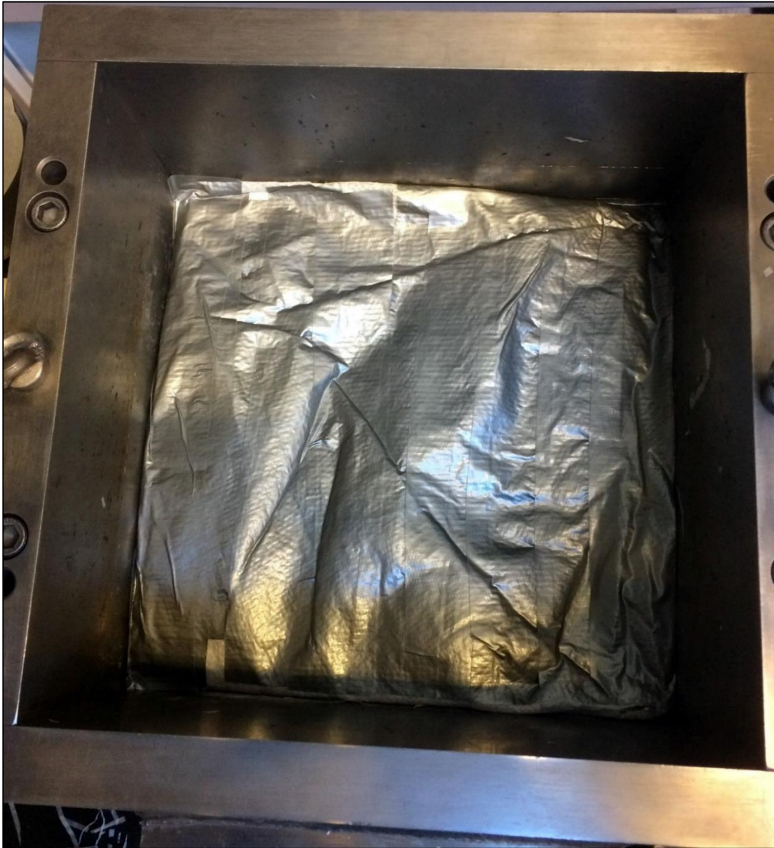
Figure 4.9: The bottom of the shear box was filled with sand in a mesh bag and covered by duct tape.
