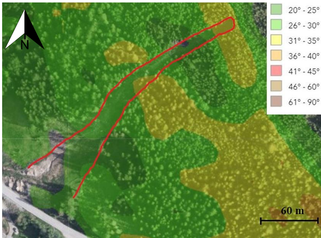
Figure 3.20 Slope gradient at location 4. Modified from NGI (2017).
