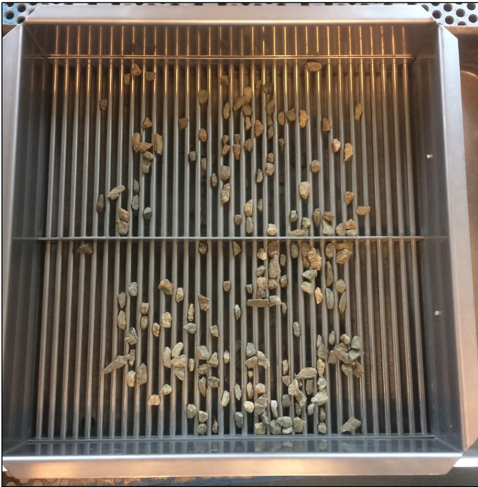
Figure 4.3: Grid sieve for determination of flakiness index
