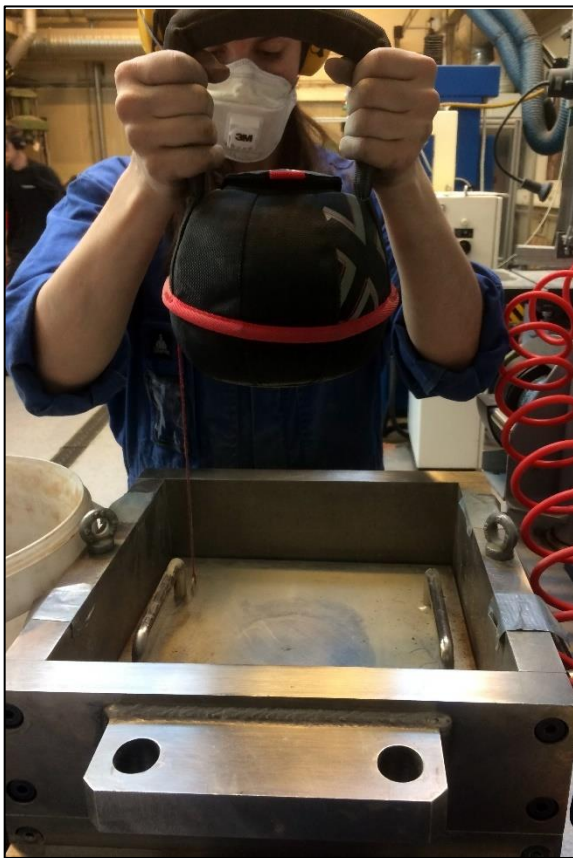
Figure 4.12: Compaction of a layer
