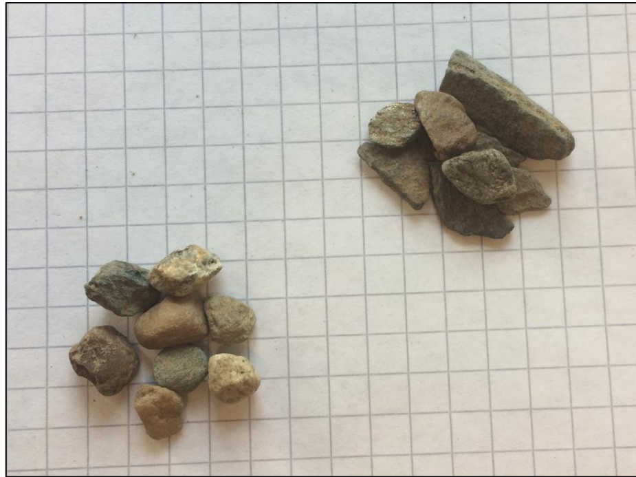
Figure 4.4: Cubical grains to the left, elongated grains to the right. The paper squares are 0.5x0.5cm.
