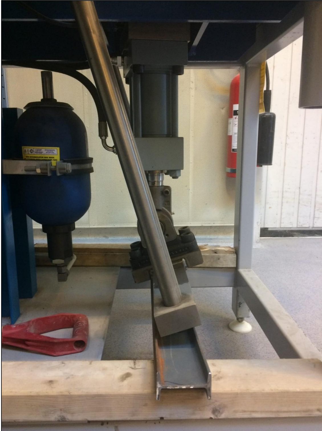
Figure 4.10: A steel beam is placed underneath the hydraulic valve.
