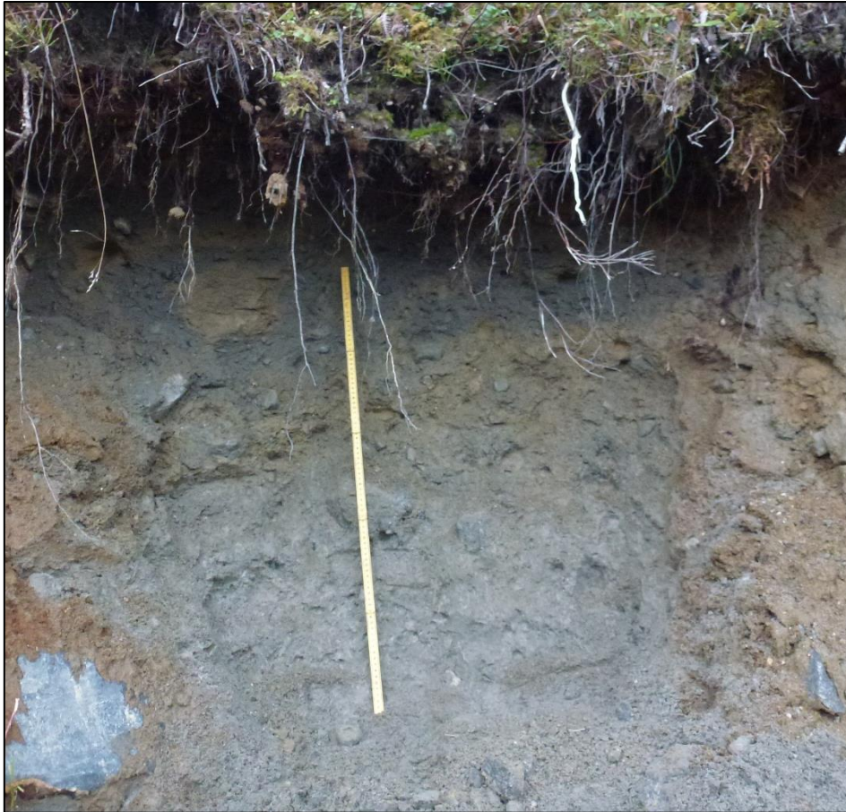
Figure 5.2 Profile at location 2B. Red colored layers in the upper part. The length of the folding ruler is 1 meter.
