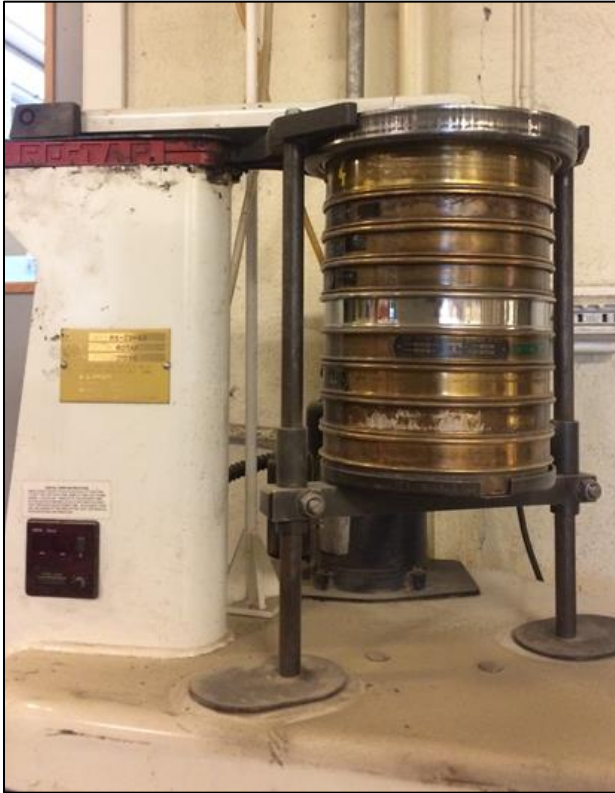
Figure 4.1 Sieving of material > 38\mu\text{m} was performed by the Rotap machine
