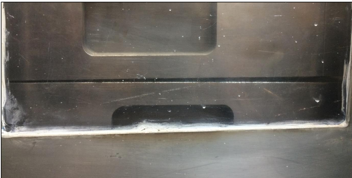
Figure 6.1: Lifting of one of the sides of the shear box.
