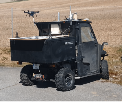
Figure 5.9: UAV landing on the FFI ground vehicle Olav
