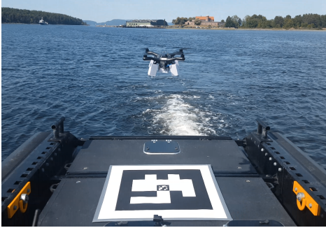
Figure 5.11: UAV landing on the FFI surface vehicle Odin
