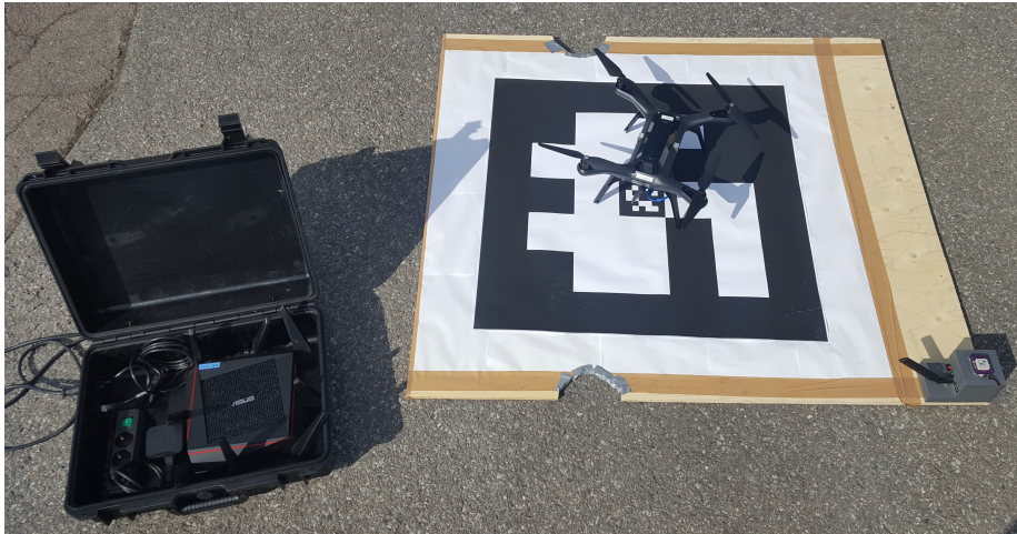
Figure 5.6: Router, UAV, CSU and landing pad Router, UAV, CSU and landing pad. Total setup for precise, autonomous landing
