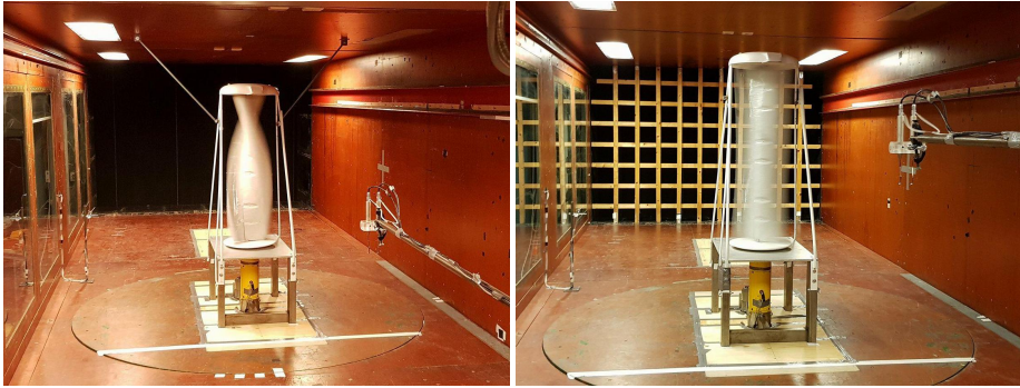
Figure 2.2: Set up in the wind tunnel. Left: Uniform inflow with additional support struts connecting the turbine to the ceiling. Right: Turbulent inflow with grid at the inlet of the test section.
