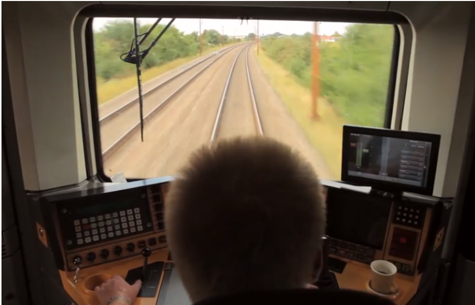
Figure 3.14.: An example of a Driver Advisory System mounted in a train cab (the extra screen on the right side.). Picture from [44]
