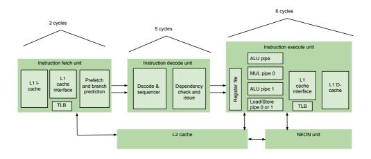
Figure 2.14: Cortex-A8 architectural overview. Adapted from the figure in [Sta13] on page 618.
