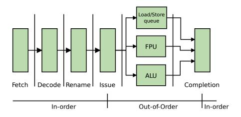
Figure 2.7: Typical architecture of an Out-of-Order processor.
