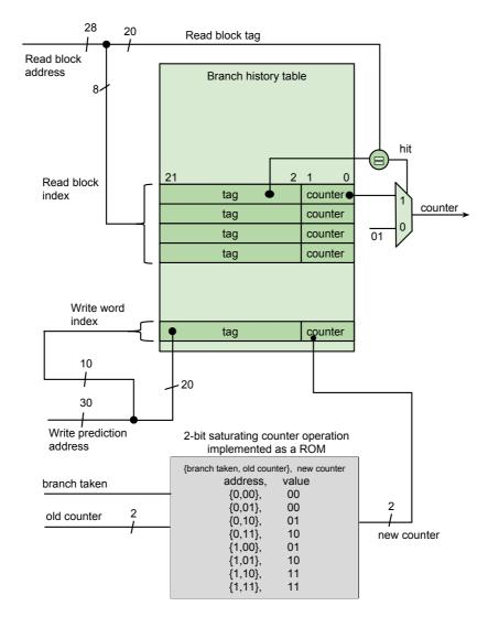
Figure 3.6: A superscalar branch history table capable of making a prediction for each of the four instructions read from the instruction cache and updating itself with one new branch each cycle. Only one tag-comparison is depicted here, but there are in fact 4 tag comparators, one for each tag in a block.
