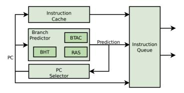
Figure 3.2: A diagram of the fetch stage showing the relationship between the instruction queue, the predictors and how the next PC is determined.
