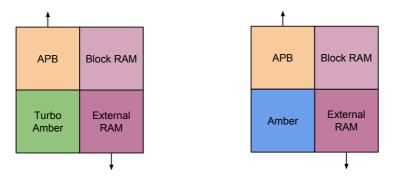
Figure 4.6: The layouts used when benchmarking Turbo Amber and Amber. Note that the APB tile and the External RAM tile are the only tiles that communicate with external peripherals.
