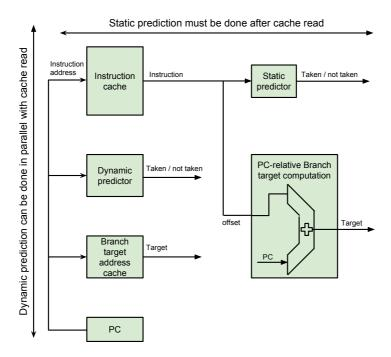
Figure 2.8: A figure demonstrating that Dynamic prediction can be done in parallel with cache read, while static prediction must be done sequentially after cache read.
