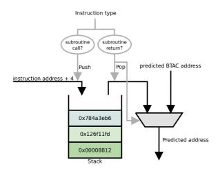
Figure 3.8: Structure of Turbo Amber's RAS
