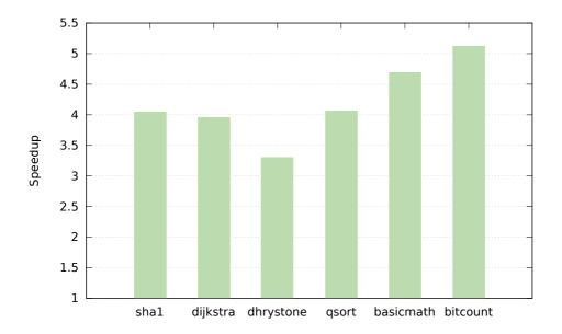
Figure 4.7: Speedups measured of Turbo Amber over Rav with caches disabled.
