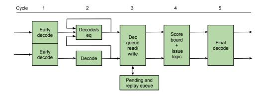
Figure 2.15: Cortex-A8 decode unit overview. Adapted from the figure in [Sta13] on page 619.
