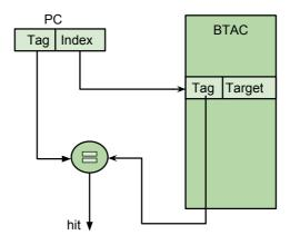
Figure 2.10: A simple view of a Branch Target Address Cache, implemented as a direct-mapped cache.
