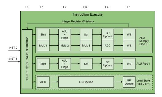
Figure 2.16: Cortex-A8 execute unit overview. Adapted from the figure in [JR07] on page 94.
