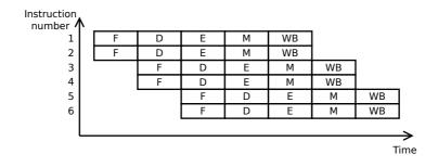
Figure 2.5: A timing diagram of a 2-way superscalar pipeline.
