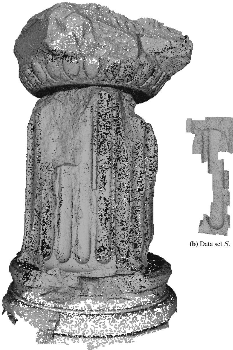
Figure 4.1: (a) Sub-sampled 3-D scan of the whole column surface. (b) Another sub-sampled 3-D scan of a part of the same column. Images are to scale relative to each other.
