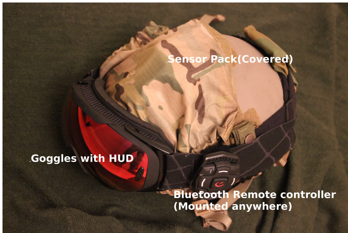
Figure 3.1: Ballistic helmet with HUD goggles, sensor module and bluetooth remote. Taken from [Moen, 2014].
