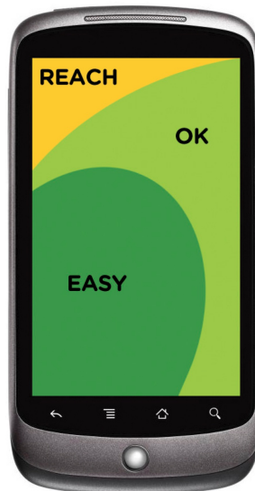
Figure 8.1: When holding a mobile phone with only the right hand, the different areas varies in how easy they are to reach with the thumb[19].
