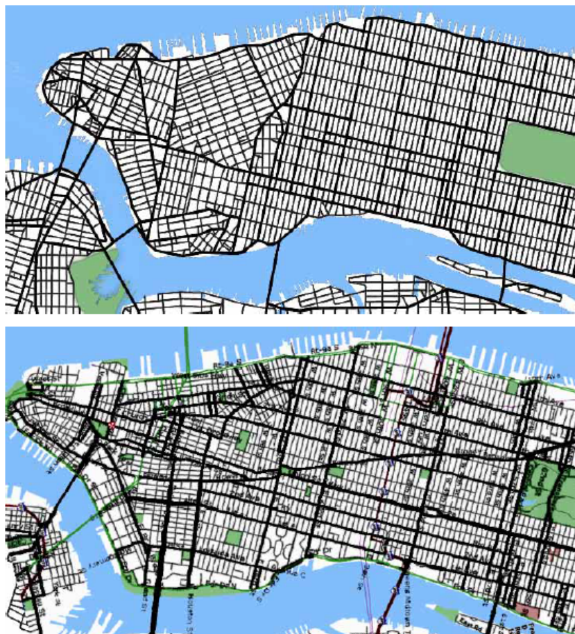
Figure 2.12: An example road network generated by an L-system. The images are adapted from [PM01]. The top image shows a road network generated inside the Manhattan island contour with specified patterns. The bottom image shows a drawn version of the actual Manhattan road network.
