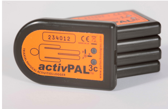
Figure 4.2: An activPAL tri-axis sensor.
