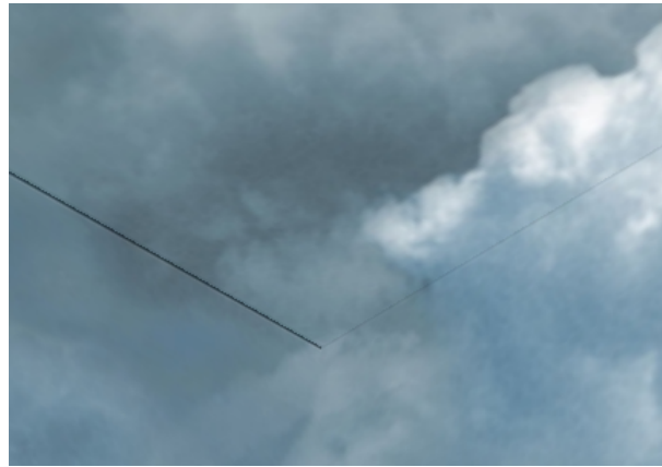
Figure 3.14: The corner of a skybox where the cube map is not aligned correctly, causing a seam.
