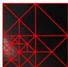
Figure 3.1 – Typical ROAM mesh
