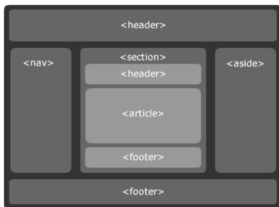
Figure 4.2: Basic HTML5 structure
