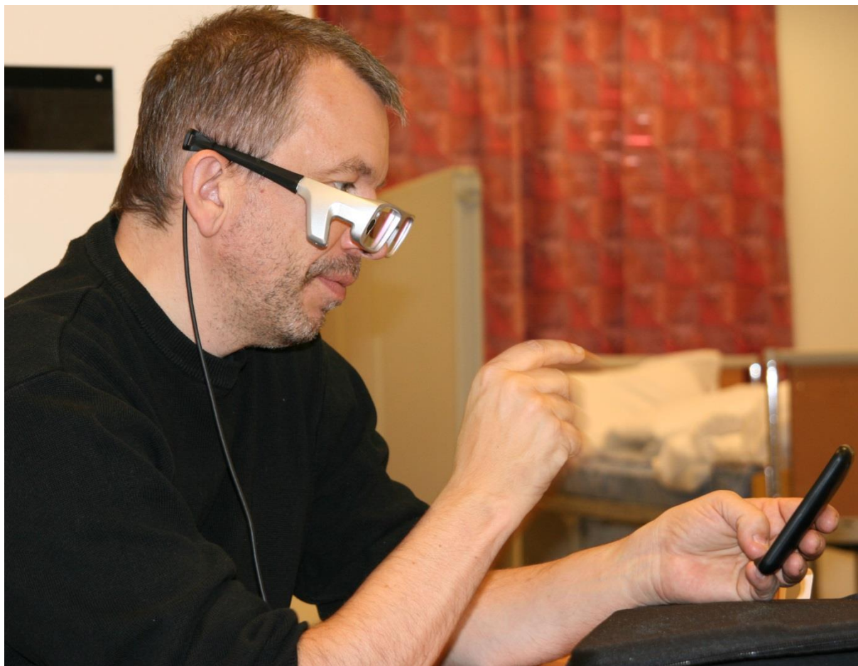
Figure 4 Tobii Glasses - eye tracker built into glasses
