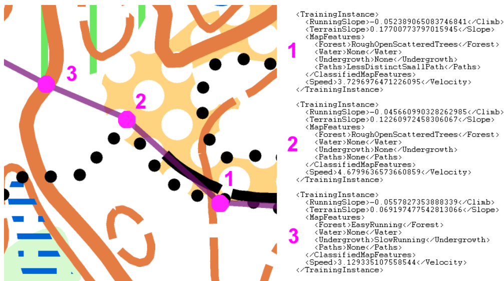
Figure 3-3: Deriving training examples from GPS track points, map and DEM. The left part of the figure shows three consecutive GPS track points superimposed on the orienteering map. (The DEM is not shown.) The right part of the figure shows the corresponding entries in the training set file. Climb and slope are computed from the DEM, while the map features are determined by looking at the appropriate coordinates of the orienteering map. Note that Speed , Running Slope and Terrain slope are based on two consecutive track points. For instance the speed for training example 2 is the average speed between track points 1 and 2. Similarly the running slope of training example 2 is the altitude difference between track points 1 and 2 divided by the distance between those points. Finally the terrain slope of training example 2 is the average terrain slope of track points 1 and 2. The map features are discrete values that cannot be averaged, so the map features of training example 2 are simply the map features present at track point 2.
