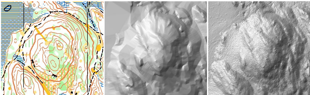
Figure 3-5: Two alternatives for obtaining a DEM. The top image shows the orienteering map. The two other images show hill shaded relief renderings of the two DEM alternatives. The first was obtained by contour interpolation, courtesy of Felix Arnet. The second was obtained from laser scans of the terrain. The renderings were created using OCAD (OCAD, 2012).
