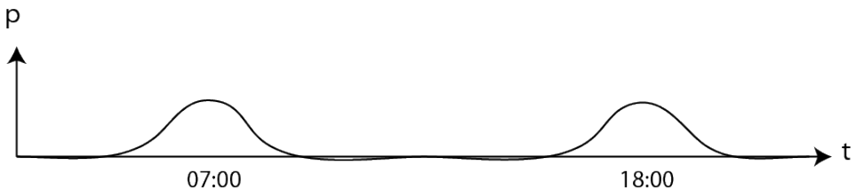
Figure 5.1: Probability distribution of time of departure for a PHEV over a 24 hour period, showing two Gaussian distributions with mean values 07:00 and 18:00
