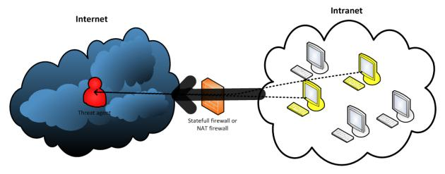
Figure 11 Illustrates that the introduction of firewalls forces adversaries to install bots that poll for new instructions to ensure continued access
