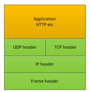
Figure 12 The Orange color illustrates that all data in the application layer of the TCP/IP stack can potentially be encrypted, and detection based on it is easy to avoid.
