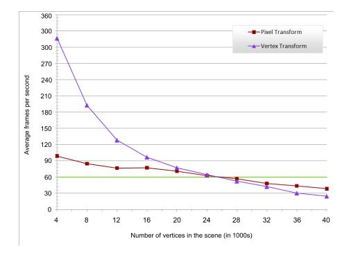
Figure 6.7: Average number of frames per second for the vertex transformation and pixel transformation code for different number of vertices.
