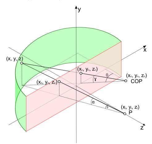
Figure 4.1: Overall view of the projection on the cylindrical part of conCave, for the pixel transformation.
