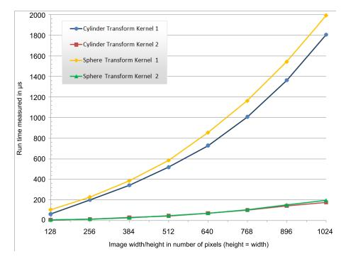
Figure 6.2: Execution time of the single transformation kernels, for different image sizes.
