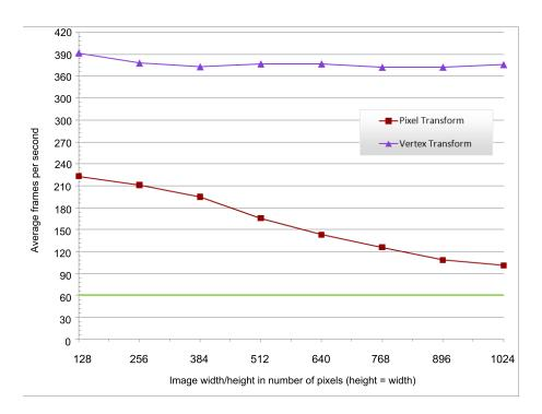
Figure 6.5: Average number of frames per second for the pixel transformation and vertex transformation code for different image sizes.
