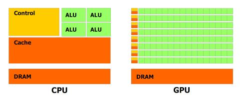
Figure 2.5: The GPU devotes more transistors to processing data, [14].
