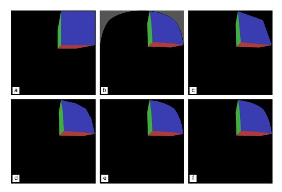
Figure 6.4: (a) Original image before transformation, (b) pixel transformation, (c)-(f) vertex transformation with 0, 1, 2, 4 and 8 additional vertices between each pair of vertices that form a line.
