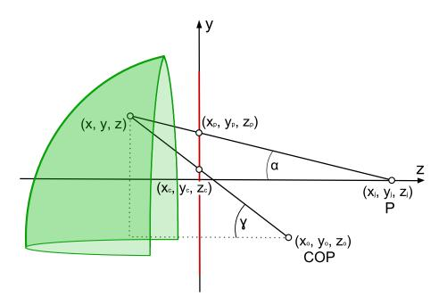
Figure 4.6: Side view of the projection on the spherical part of conCave, for the pixel transformation.
