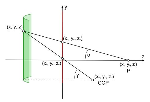
Figure 4.3: Side view of the projection on the cylindrical part of conCave, for the pixel transformation.
