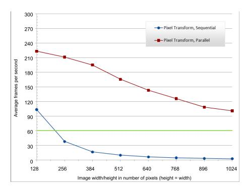
Figure 6.3: Average number of frames per second for the sequential and parallel pixel transformation code, for different image sizes.
