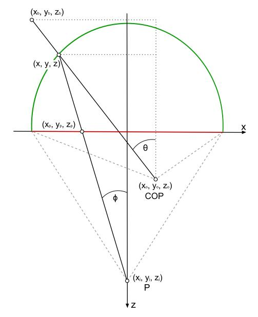
Figure 4.7: Top view of the projection on the cylindrical part of conCave, for the vertex transformation.
