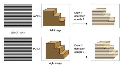
Figure 5.2: Rendering the stereo pair using a stencil mask.
