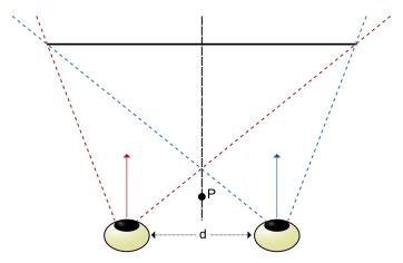
Figure 2.4: Creating a stereo pair from a reference point P and distance d between two eye/camera positions.
