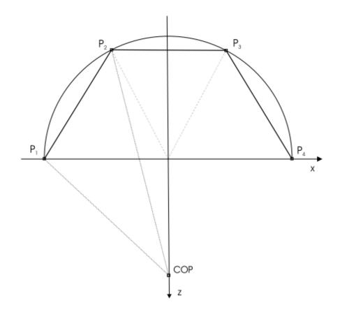
Figure 3.1: Plane approximation of the cylindrical part of the conCave surface, using three segments (seen from above). Image taken from [1].
