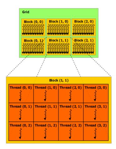
Figure A.1: CUDA thread hierarchy, taken from [13] with permission from NVIDIA.
