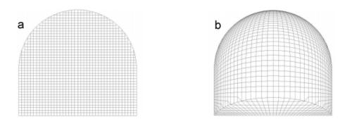
Figure 3.2: (a) Grid placed in front of the conCave surface before transformation, (b) grid after transformation (seen from the front). Images taken from [2].
