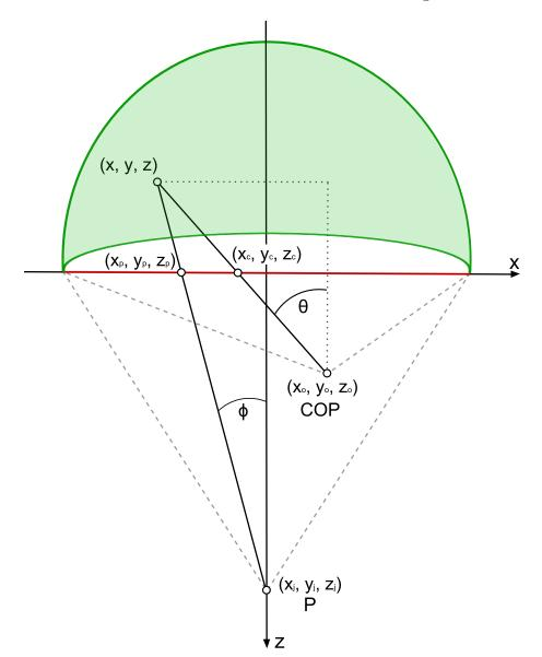
Figure 4.5: Top view of the projection on the spherical part of conCave, for the pixel transformation.
