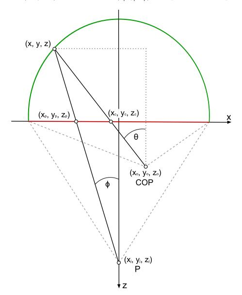
Figure 4.2: Top view of the projection on the cylindrical part of conCave, for the pixel transformation.
