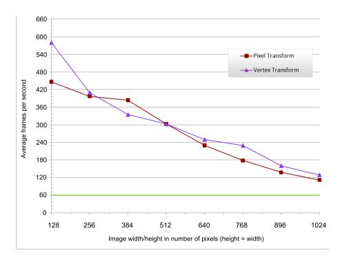
Figure 6.8: Average number of frames per second for the vertex transformation and pixel transformation code for image sizes, and with dynamic addition of vertices.
