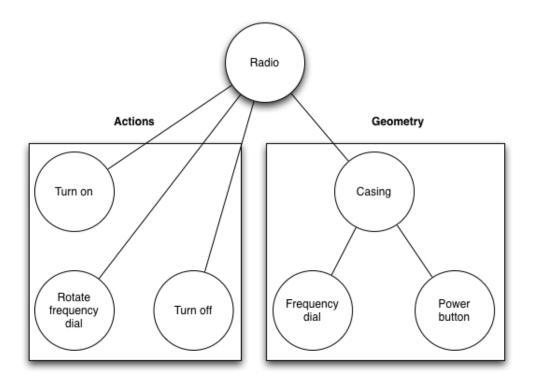
Figure 2.3: Radio in Fig 2.2 represented as a tree
