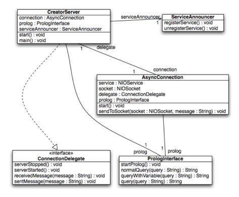
Figure 3.3: Simplified class diagram of the server architecture.
