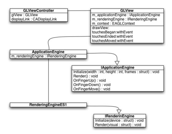
Figure 3.6: The basic structure of our OpenGL rendering engine.
