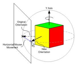
Figure 2.6: Translating 2D coordinates into 3D coordinates through the use of an arcball.
