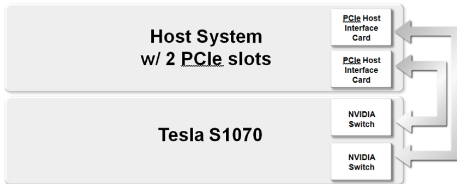
Figure 2.11: NVIDIA Tesla S1070 connection configuration (from [32], used with permission)
