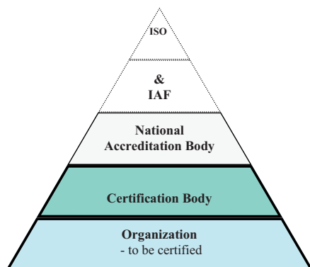
Figure 2.2. A substantial pyramid of trust, topped by ISO and IAF, form a backdrop for a certified organization, in effect validating the certificate.
