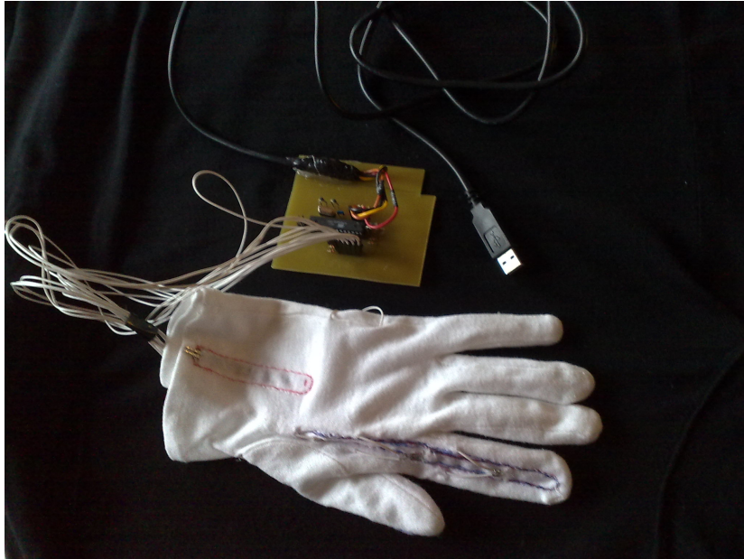
Figure 4: Data glove and Printed Circuit Board w/USB
