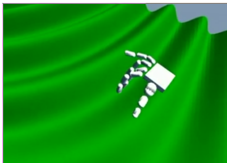
Figure 2: Hand of collision primitives simulating haptic feedback from rough surface
