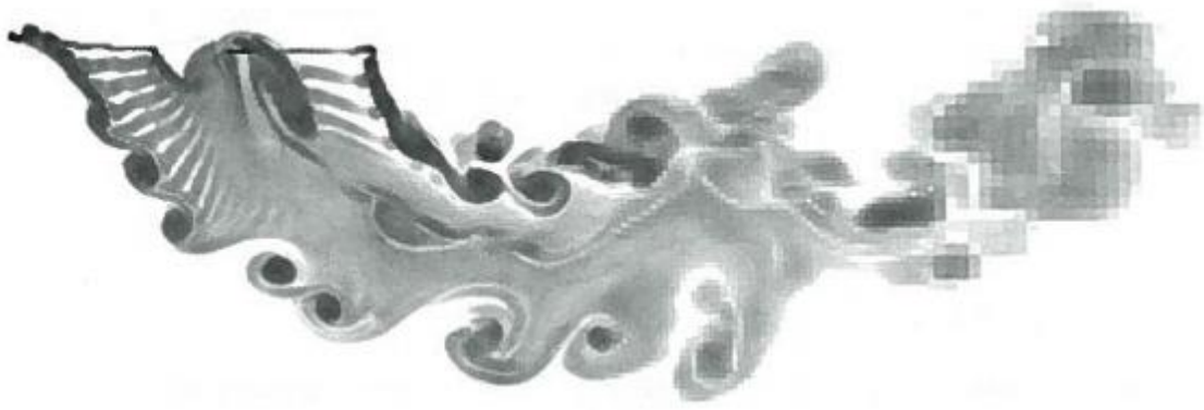
Figure 2.9: Vorticity in the rotor wake of a helicopter modeled by VTM. Note how the grid resolution is detailed near the rotors and gradually less detailed further away. Source: [8, p. 779]
