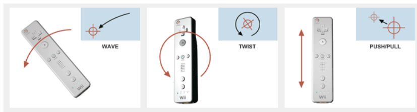
Figure 2.4: Wiimote motion sensing
