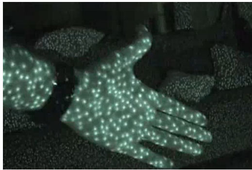
Figure 3.4: A hand with lights emitted from Kinect taken with a night vision camera
