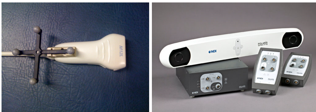
Figure 2.4: GE M12L linear array probe (GE Healthcare, Waukesha, Wisconsin, USA) with tracking frame and Polaris Spectra optical tracking system (Northern Digital, Waterloo, Canada) (Photo of Polaris Spectra used with permission from Northern Digital Inc.)
