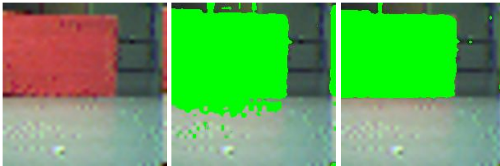
(a) Original image, red box. (b) Thresholding using max . Some gray pixels are erroneously labeled as red. (c) Thresholding using the r:g ratio of each pixel, \frac{r}{g} \geq 1.3 .
