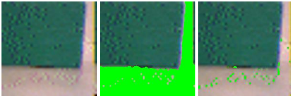
(g) Original image, a green box (no pixels should be marked as red). (h) Thresholding using max . Almost all gray pixels are marked red. (i) Thresholding using the r:g ratio of each pixel, \frac{r}{g} \geq 1.3 . A few gray pixels are marked red.
