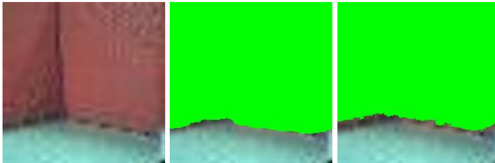
(d) Original image, red boxes covered by shadow. (e) Thresholding using max . (f) Thresholding using the r:g ratio of each pixel, \frac{r}{g} \geq 1.3 .
