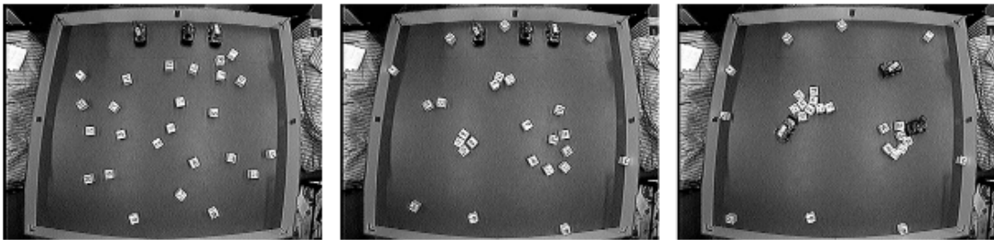
Figure 2.11: Clustering of boxes by DidaBots. Courtesy of the Artificial Intelligence Lab, University of Zurich.
