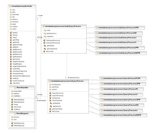
Figure 5.6: A class diagram for the simulation.query package
