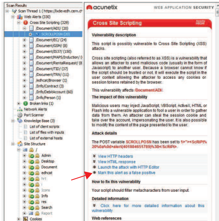
Figure 4.1: By first selecting a false-positive vulnerability, and then clicking on “Mark this alert as a false positive” (indicated by the red arrow), a false-positive is marked. The specific false-positive won’t be treated as a vulnerability next time Acunetix WVS encounters it on the respective Web site/application.
