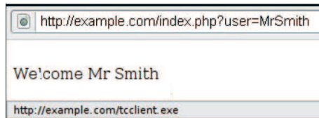
Figure A.1: A Web application potentially vulnerable to XSS. This figure is adapted from OWASP Testing Guide V3.0 [102].
