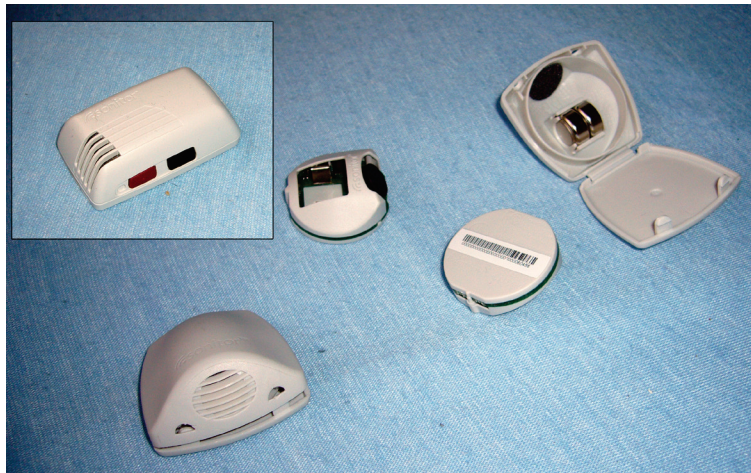
Figure 3 Various Sonitor Tags. E-Tag (inset), two P-Tag cores and two P-Tag shells (open and closed)
