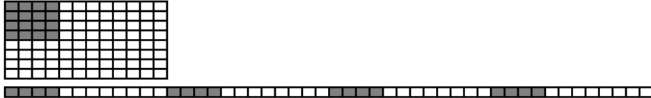
Figure 3.3: Illustration of how a 4x4 block might be distributed in memory.
