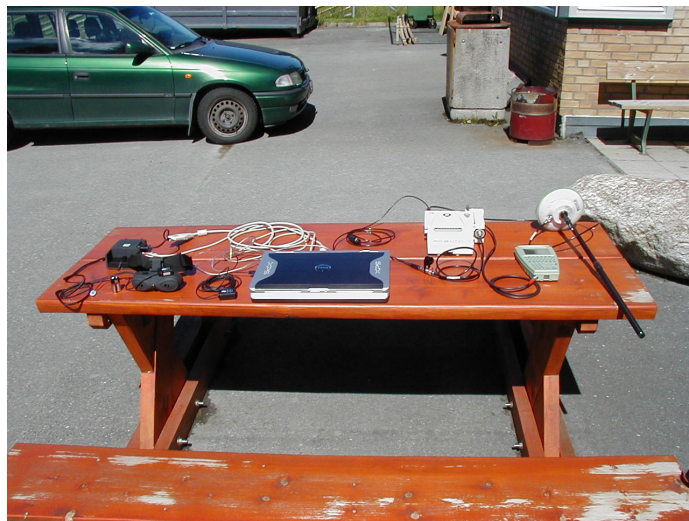
Figure 8.3: All the equipment connected together, but not packed. From left: HMD with Wireless InertiaCube3 and battery, Wireless InertiaCube3 receiver, laptop, GSM antennae, DGPS core unit, DGPS remote control and GNSS antennae.
