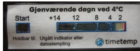
Figure 2 Chemical sensor (TimeTemp 2008)
