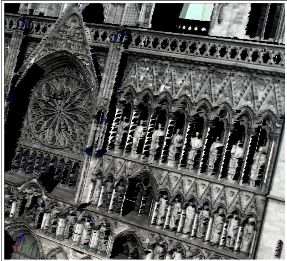
Figure 3.7: Point cloud triangulated by RiSCAN PRO.
