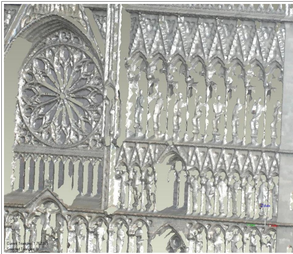
Figure 3.8: Point cloud triangulated by Geomagic Studio.
