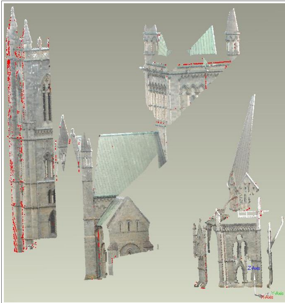
Figure 3.4: Geomagic Studio's plane based noise reduction algorithm in progress.
