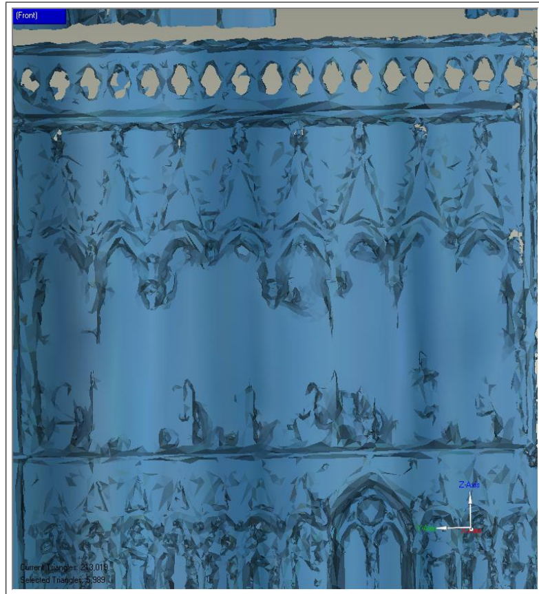
Figure 3.14: Automatic hole filling of sculptures with Geomagic Studio. Compare to Figure 3.13 and Figure 3.15.
