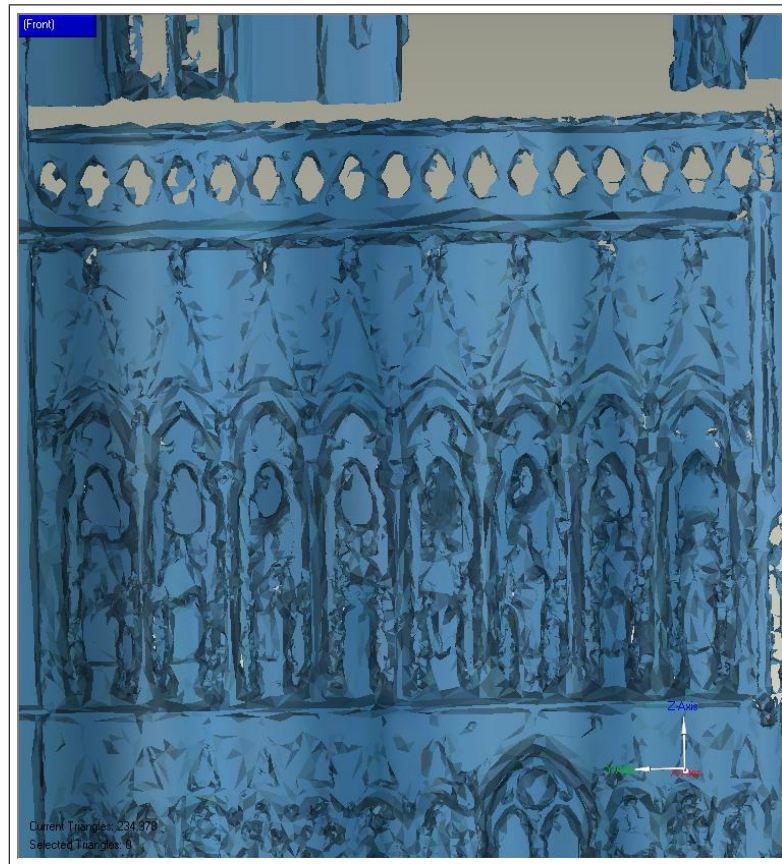
Figure 3.15: Manual hole filling of sculptures. Compare to Figure 3.13 and Figure 3.14.
