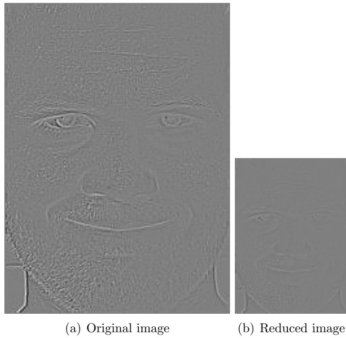
Figure 3.4: Input image edge detected, then scaled by ordinary algorithm.
