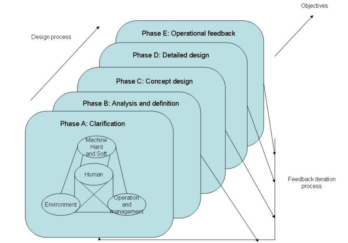
**Figure 5-13 Ergonomic approach to system designs from ISO 11064: Ergonomic design of control centers, Part 1: Principles for the design of control centers (2000). [19]**
