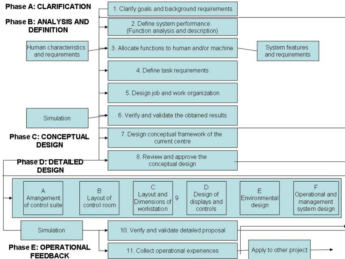
**Figure 5-12 Ergonomic design process for control centers from ISO 11064: Ergonomic design of control centers, Part 1: Principles for the design of control centers (2000) [19]**
