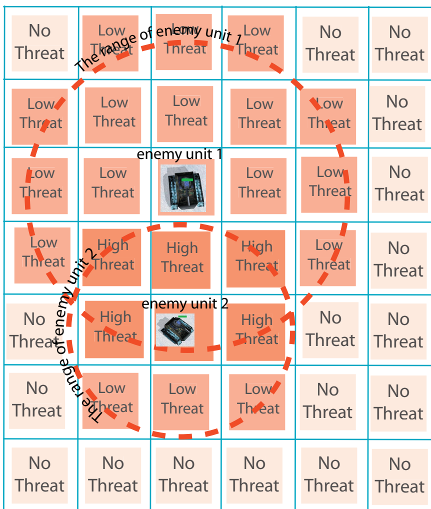
Figure 14: An illustration of an excerpt from a threat map with various threat values determined by nearby enemy units. The damage that the units are able to deal decides the level of threat, and their maximum attack range determines which fields the damage value is added to. Note the “High Threat” areas within reach of both units.
