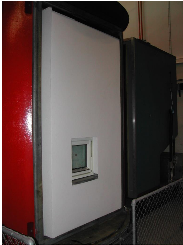
Figure 2. A large test area installed in SINTEF's climate simulator according to NT Build 495:2000 [17].
