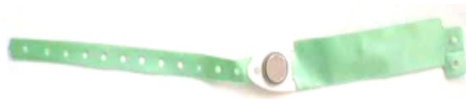
Fig.5.9: Patient ID bracelet with iButton holder (Dallas Industrial Data Inc).
