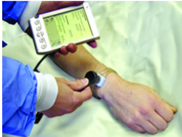
Fig.5.10: iButton on patient bracelet (OneTouch Technologies Corporation).
