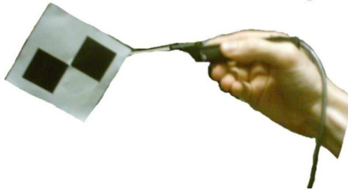
Figure 5.9: The tracked pen with a 2 \times 2 chessboard pattern attached. The pattern has to be placed with the center at the tip of the pen. Calibration is performed by slowly moving the pen in front of the camera while both the head and pen are being tracked.
