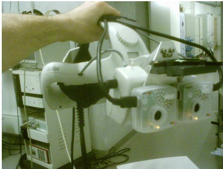
Figure 4.4: An Augmented Reality enhanced CardioView HMD. The cameras are mounted upside down in front of the displays of the HMD to reduce the parallax error. The tracker is located above the cameras to be easily seen by the tracking system located in the ceiling.
