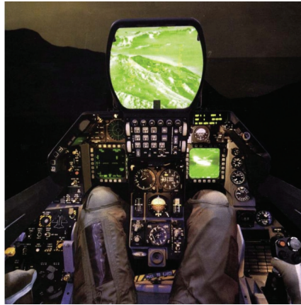
Figure 2.11: HUD projecting a FLIR video image
