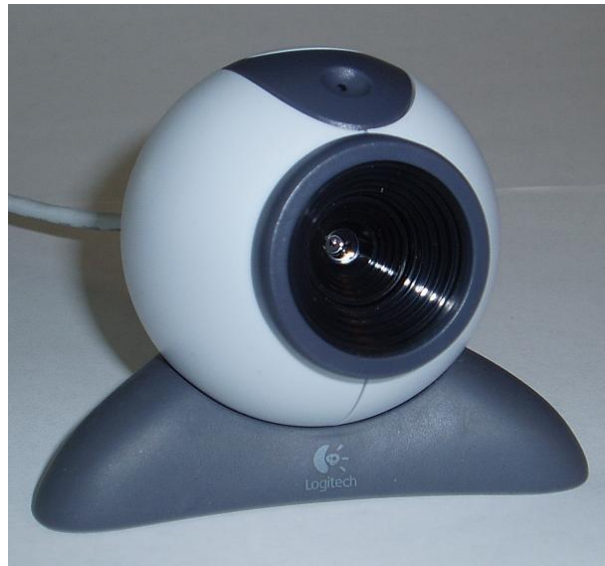
Figure 6.1: The camera: Logitech QuickCam Messenger.
