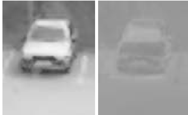
Figure 6.3: The models used for the car scene after trained with 7799 images, to the left is the expectation value for each pixel and to the right is the standard deviation for each pixel.
