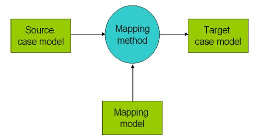
Figure 5.1: Mapping method uses a mapping (domain) model to construct target model (adapted from [Ste91])
